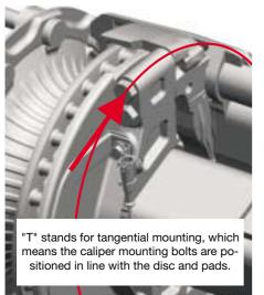
The SB 4345 T will be used for axle loads of 11t and 12 t in future.
