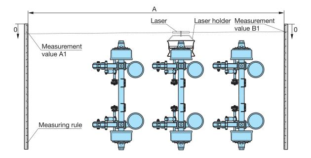
The measurement must be performed on both sides of the axle. The measurement values are then added together. The total of the values is the toe-in/toe-out value of the axle and must be within the permitted tolerance range.
