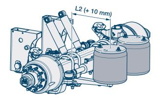
The following new air bags with Ø 360 mm are being introduced for positively steering axles with underslung AL2 air suspension of axle series N/K/M...ALUL:
