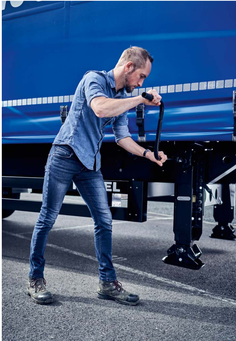
The BPW drawbar supports in use
